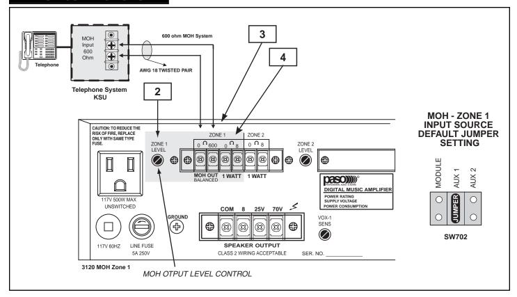
Fig. 25 - Rear Panel MOH Connection Diagram
